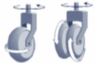
Figure 6b. Single wheel casters pivot on the wheel surface, leading to increased force due to friction and wheel surface damage. Twin wheeled casters (right) reduce friction and wheel damage by rolling when the caster is rotated.
