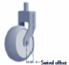
Figure 6b. Single wheel casters pivot on the wheel surface, leading to increased force due to friction and wheel surface damage. Twin wheeled casters (right) reduce friction and wheel damage by rolling when the caster is rotated.
