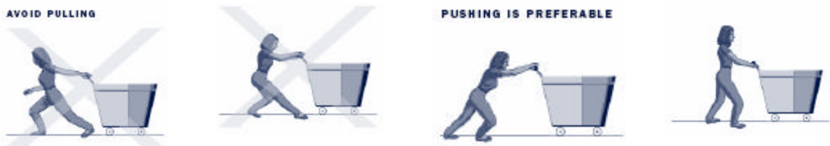
Figure 2. Given the choice between pushing and pulling, a task should be designed for pushing.
